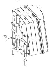
Fig. 2: Removing the wall/tube retaining bracket
