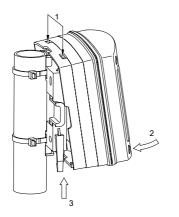
Fig. 5: Suspend the peristaltic pump and fix in place
