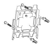
Fig. 3: Screw the wall/tube retaining bracket in place using the washers
