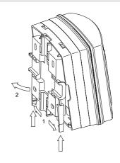
Fig. 4: Removing the wall/tube retaining bracket
